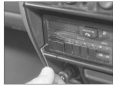
22.2 Unscrewing the securing pins from the radio/cassette player
